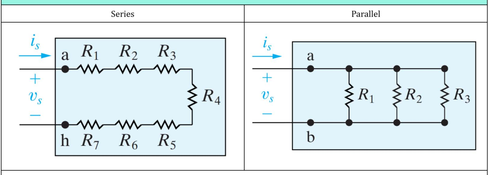
Both circuits above can be simplified to a circuit with one equivalent resistor
