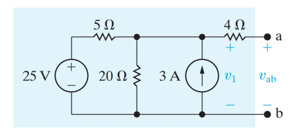
A Norton equivalent circuit consists of an independent current source in parallel with the Norton equivalent resistor.
